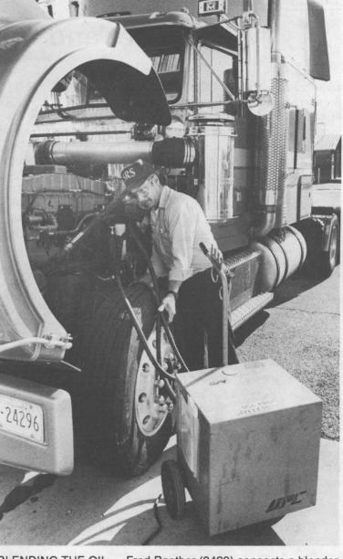
BLENDING THE OIL — Fred Raether (3423) connects a blender that takes oil from the crankcase of this DOE tractor, filters it, and mixes it with the tractor's diesel fuel. This use of motor oil, approved by the engine manufacturer and certified by the EPA, saves the cost and the environmental impact of disposing of it as hazardous waste after an oil change.
